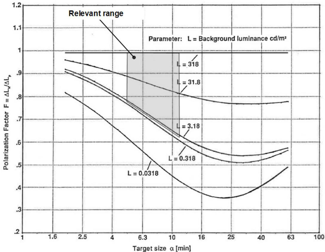
**Figure A.11: The polarization factor as a function of the object size and the background luminance.**
