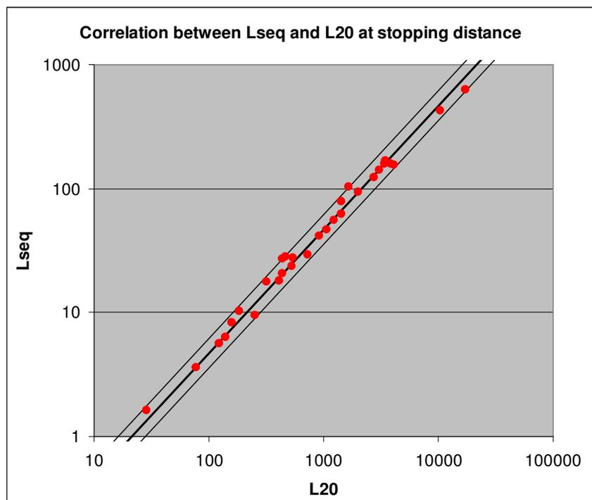
**Figure A.13: Correlation between of  $L_{seq}$  and  $L_{20}$  for 15 tunnels in Norway measured in both directions.**
