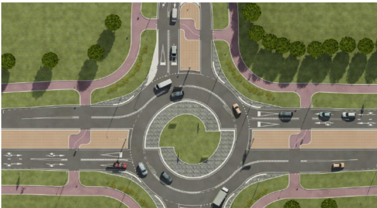
Figure 46: Standard layout of a turbo roundabout
