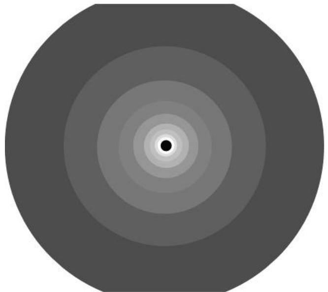
Figure 4: Varying weights in the polar diagram for the determination of L_{seq} .
