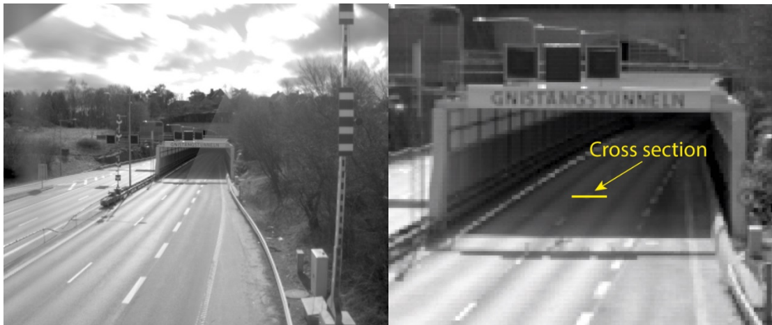
Figure 22. Luminance image (left) with a superimposed veiling luminance in the right half of the image. Magnification of the tunnel entrance (right) with a line marking the position used for contrast calculations.
