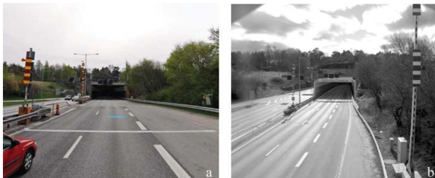
Figure 28. Comparison of field of view from different height above the road. a) Height is approximately 2 m and in the middle of right lane. b) Height is 7 m and to the right of the road.
