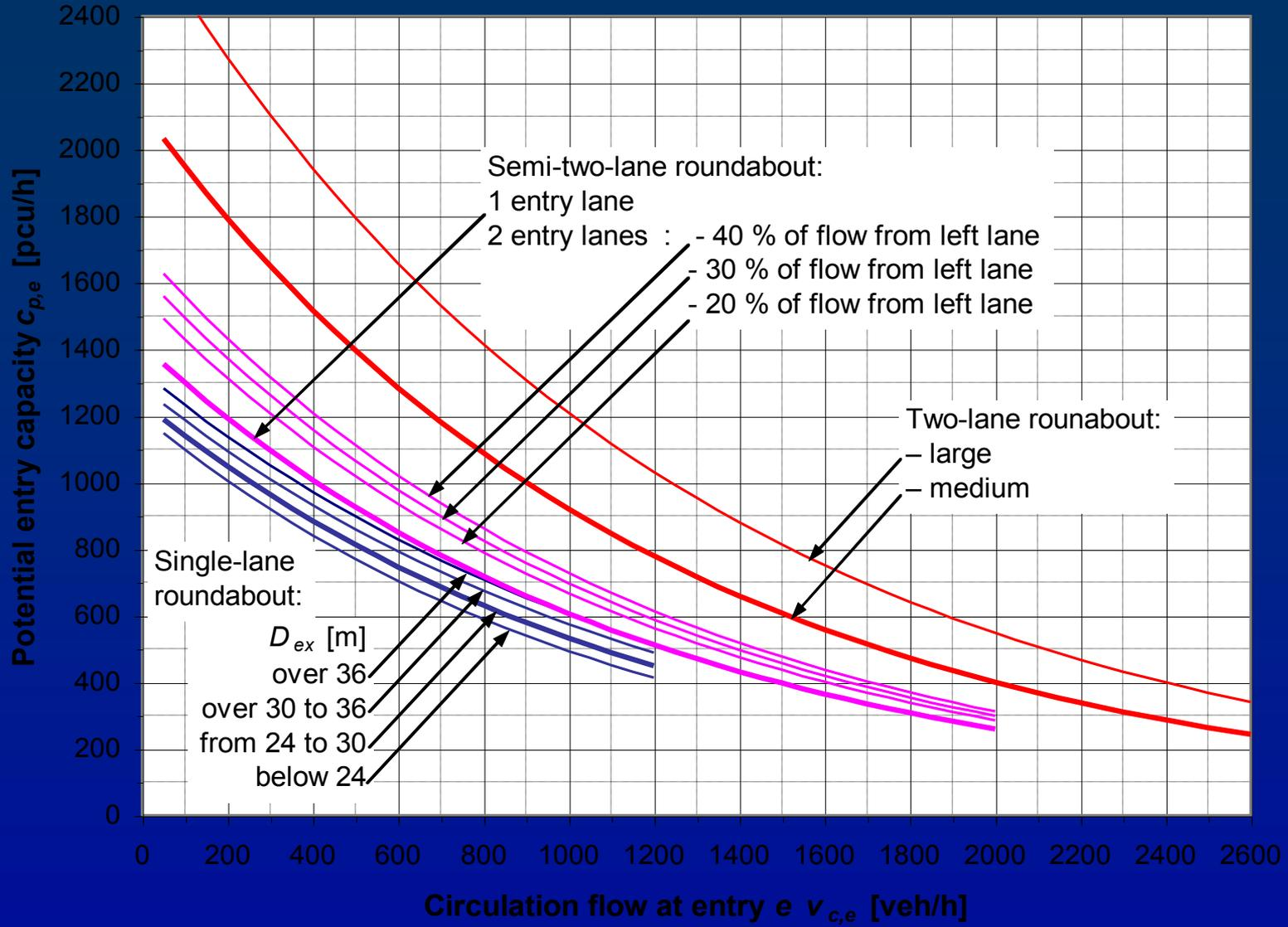
**Comparison of initial capacities on minor entries of a one-lane, two-lane and semi-two-lane roundabout**
