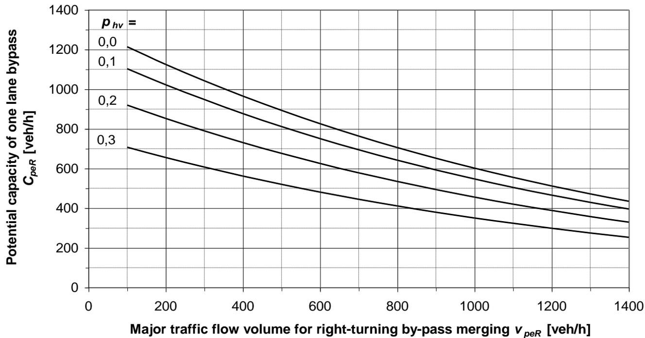
Fig. 8 Potential capacity of one-lane bypass
