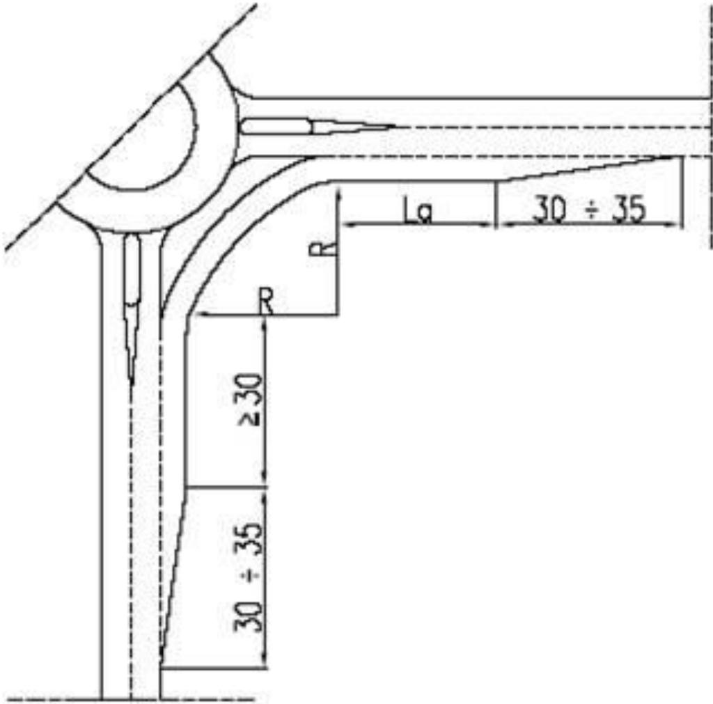
Polish guidelines for designing roundabouts recommend one simple type of right-turn by-pass. The design should include even short merging lane ( $>30$  m) parallel to the main exit lane for safety of merging and **separate right-turning lane at the entry**.
