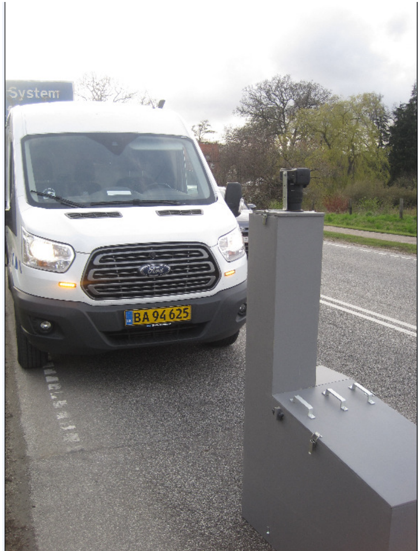
Figure 3: The instrument placed on the road with protection by a vehicle with a flashing yellow arrow on a trailer.
