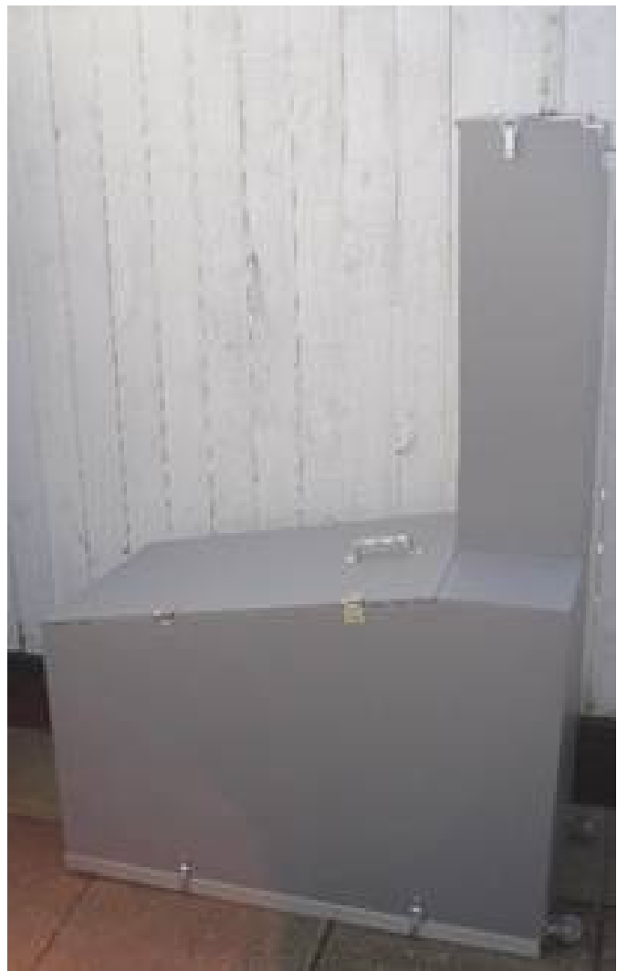
Figure 9: The prototype instrument with the camera mount at the top.
