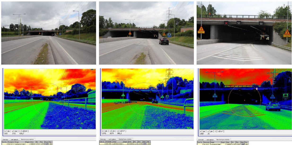
Fig.7: Photos taken on 2013/07/02 at the northern entrance of Häggvik tunnel. On the bottom row, showing photos taken using an LMK luminance camera, the L20 circle of 2X10^0 is positioned in an attempt to gather data about the influence of the light levels changing towards the tunnel entrance.
