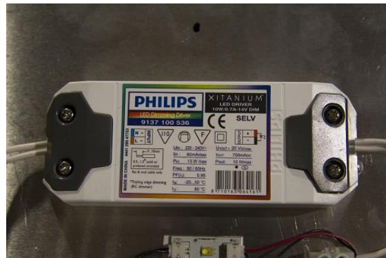
Fig.20: Xitanium 150W Programmable LED driver for the Fortimo drivers (one for every fixture). Fig.21: Xitanium LED Driver 10W/0.70A-14V DIM for the small LED.
