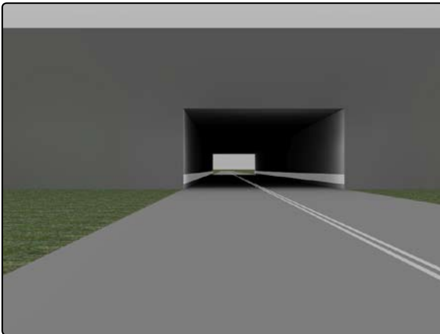
Figure 24: Lighting approach No. 2: Luminous band
