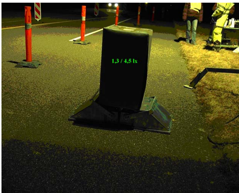
Fig. 8. Measured vertical illuminance on the box without/with bypassing car with low beam headlights.
