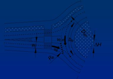
Illustration of roundabout geometric and traffic parameters
