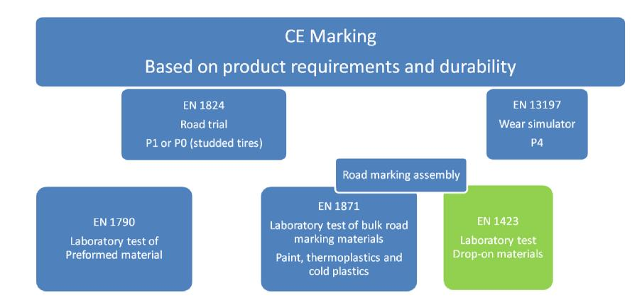
The CE marking will be placed on the base product, but are tested on the assembly
