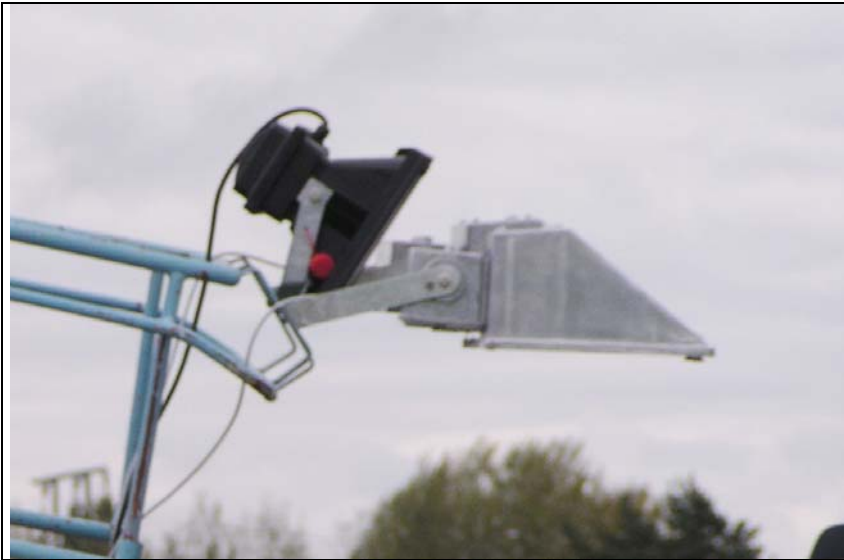
Figure 12. Two types of luminaires to demonstrate the traditional lighting method (dark luminaire) and an alternative method (light luminaire)
