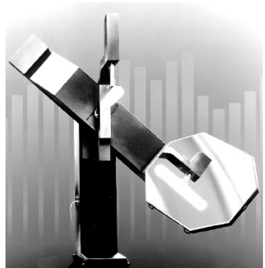
Figure 33: A rotating mirror light distribution photometer.
