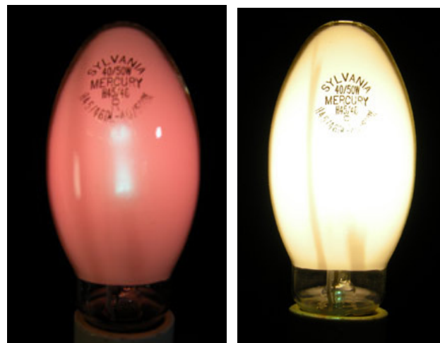
Figure B.23: A mercury lamp at start up (left) and warm (right).
