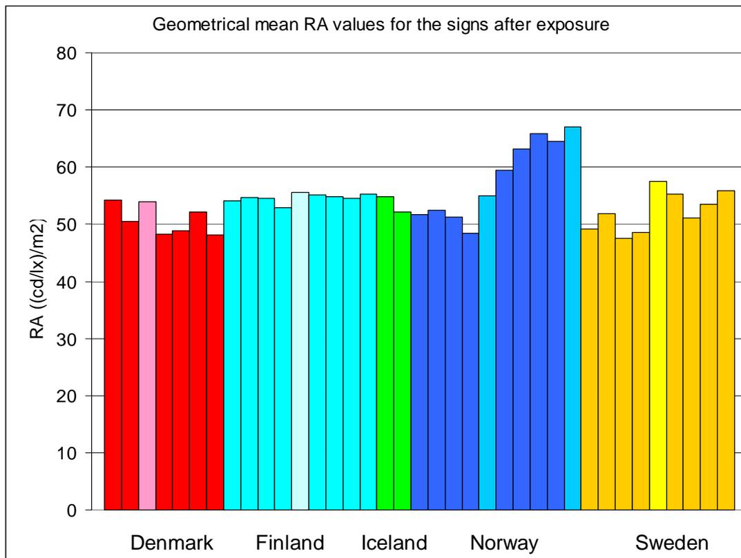
**Figure 8: Geometrical mean  $R_A$  values ( $\text{cd}\cdot\text{lx}^{-1}\cdot\text{m}^{-2}$ ) for the test and reference signs in the initial condition**
