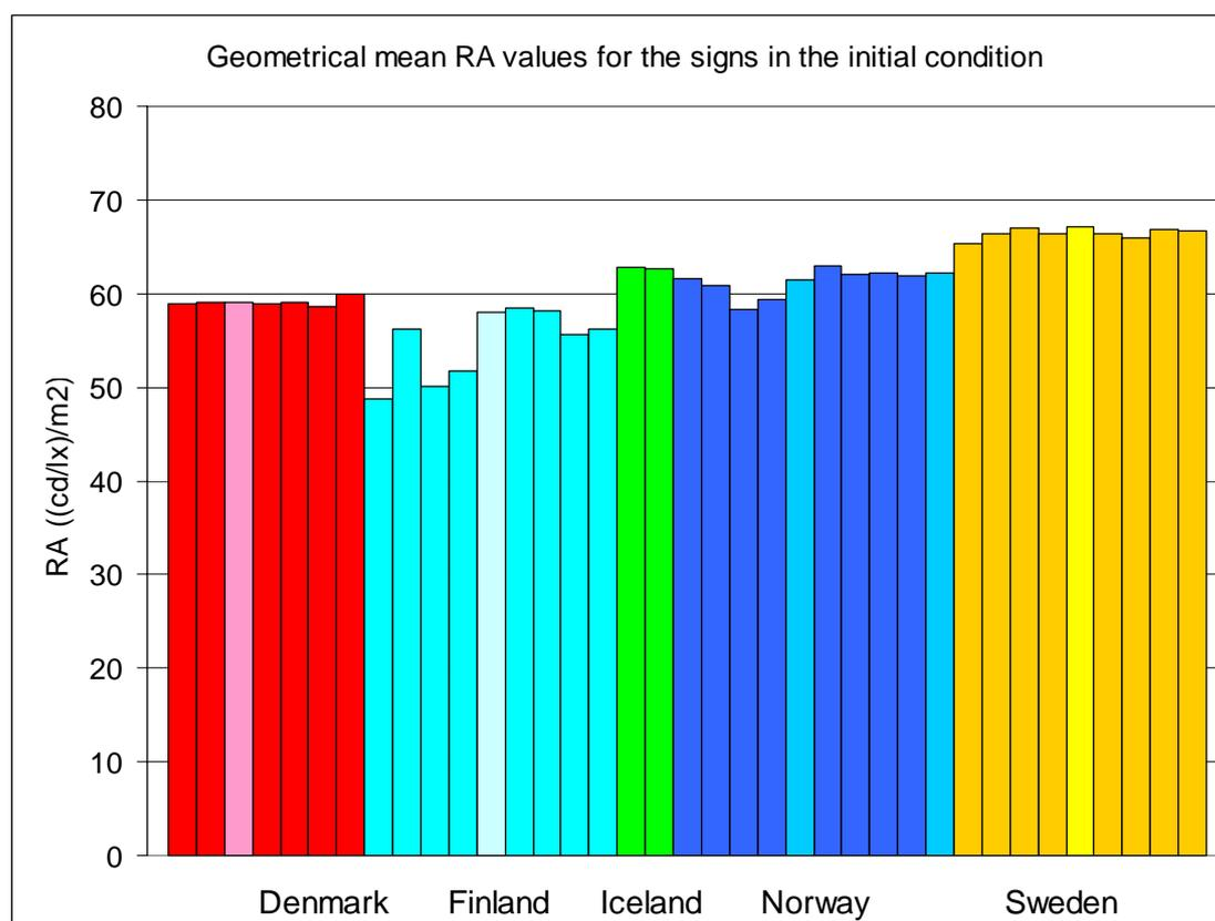
Figure 7: Geometrical mean  $R_A$  values ( $\text{cd}\cdot\text{lx}^{-1}\cdot\text{m}^{-2}$ ) for the test and reference signs in the initial condition.
