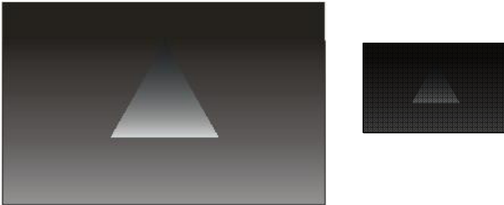
Figure 26: Both luminance and apparent size decrease with distance to a line and, therefore, visibility decreases strongly with distance.
