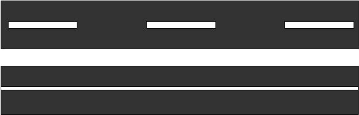
Figure 25: The effective width of a broken line (top) is the width of a continuous line with the same surface area (bottom).
