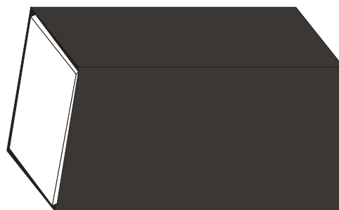
Figure D.18: Calibration block with a white tilted surface.
