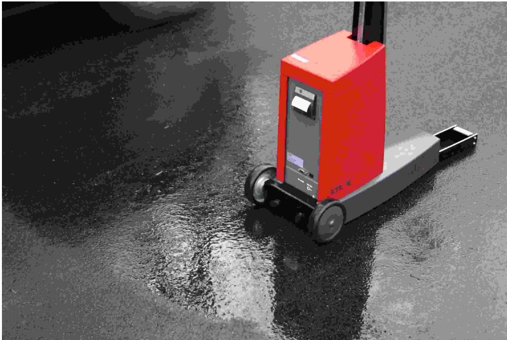
Figure C.7: A handheld retroreflectometer using the CEN 30 m geometry with modification to provide the specular reflection value instead of the retroreflection value.
