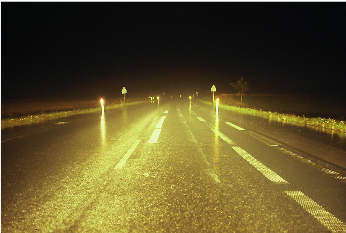
Figure 15: Road markings at a road trial site in the dry condition (top) and during a light rain (bottom).
