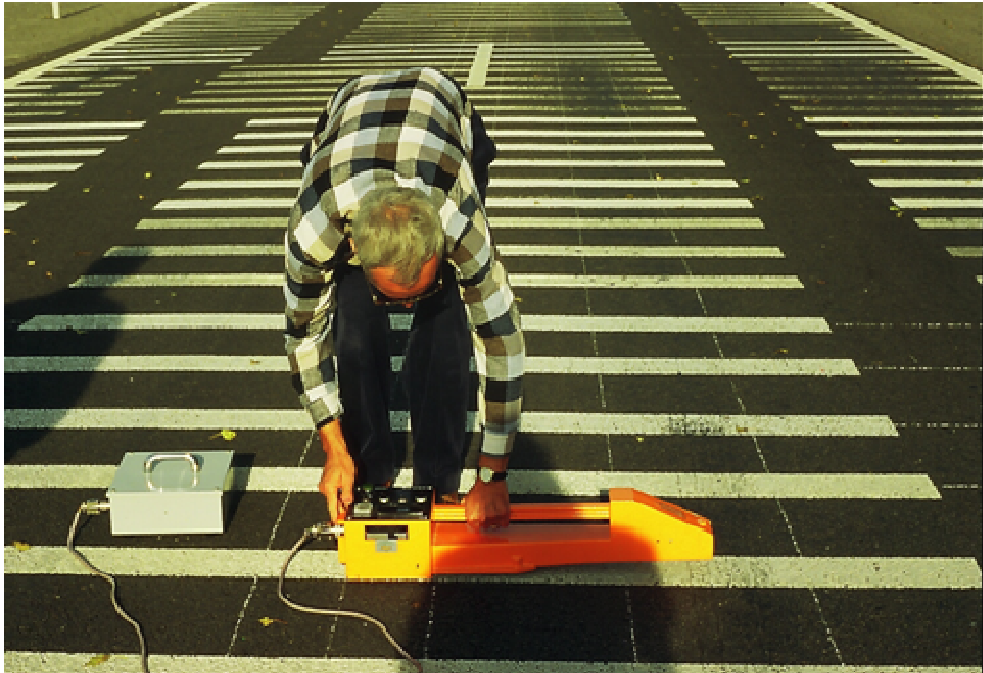
Figure D.7: Another early type of retroreflectometer.
