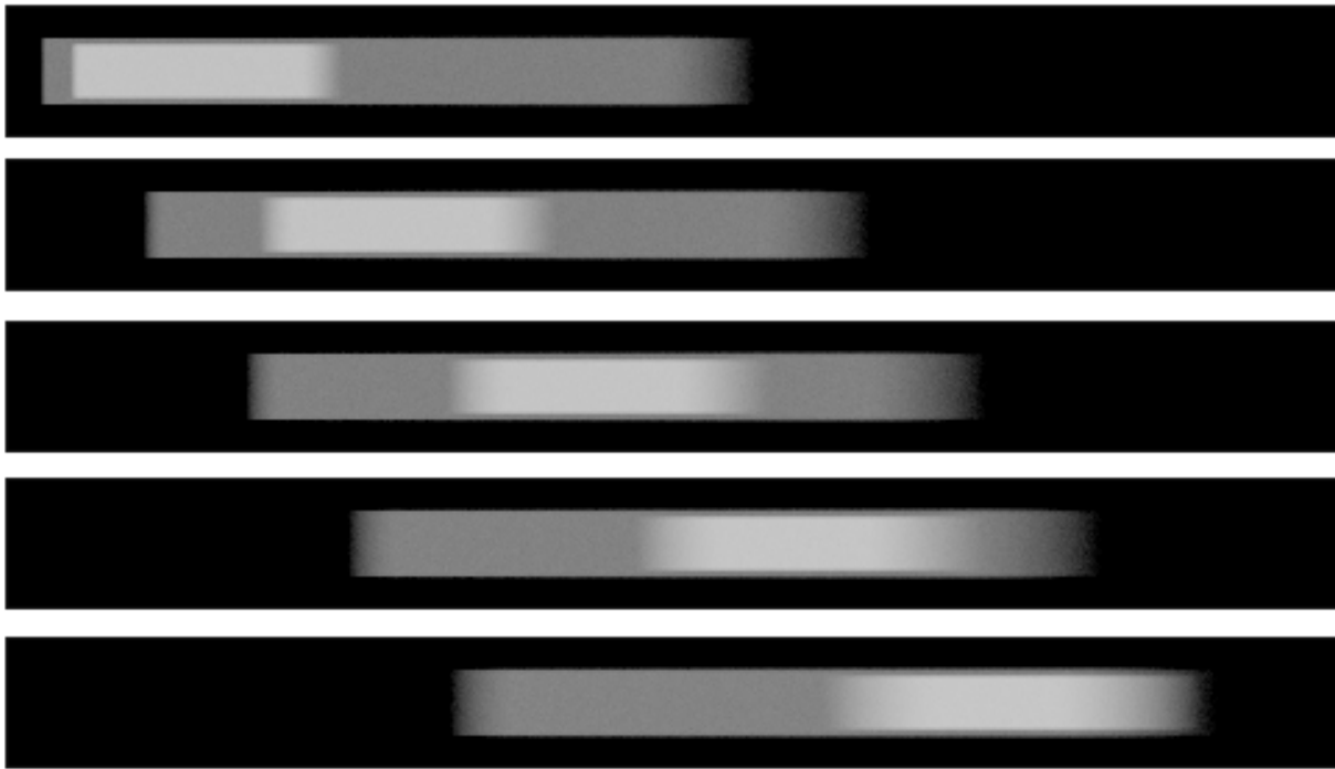
Figure D.16: Movements of the illuminated and the measured fields with lift of the retroreflector in uniform steps.
