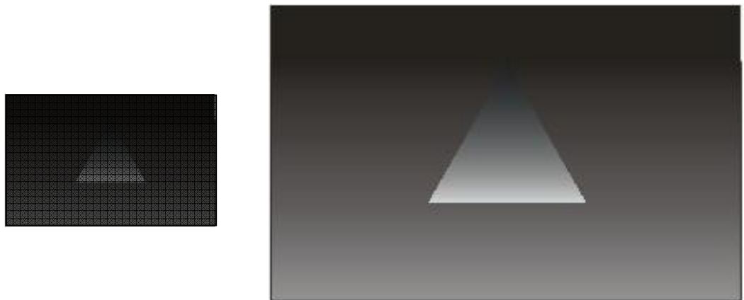
Figure F.4: A line shown at a long distance (left) and a shorter distance (right) illustrating that both luminance and apparent size increase, when approaching a line.
