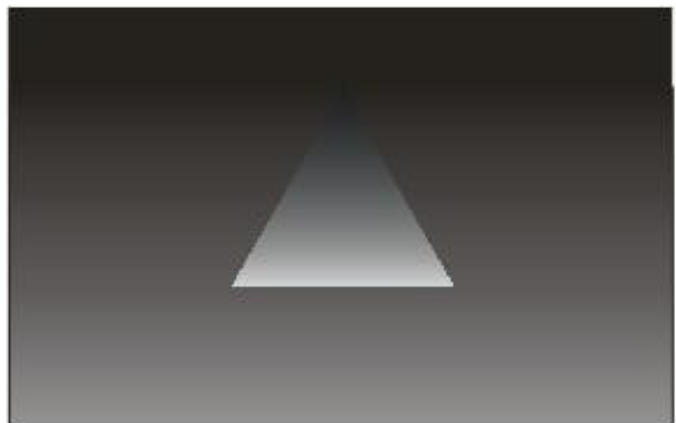
Figure 24: A longitudinal road marking when seen by the driver of a vehicle and illuminated by the headlamps of the vehicle.
