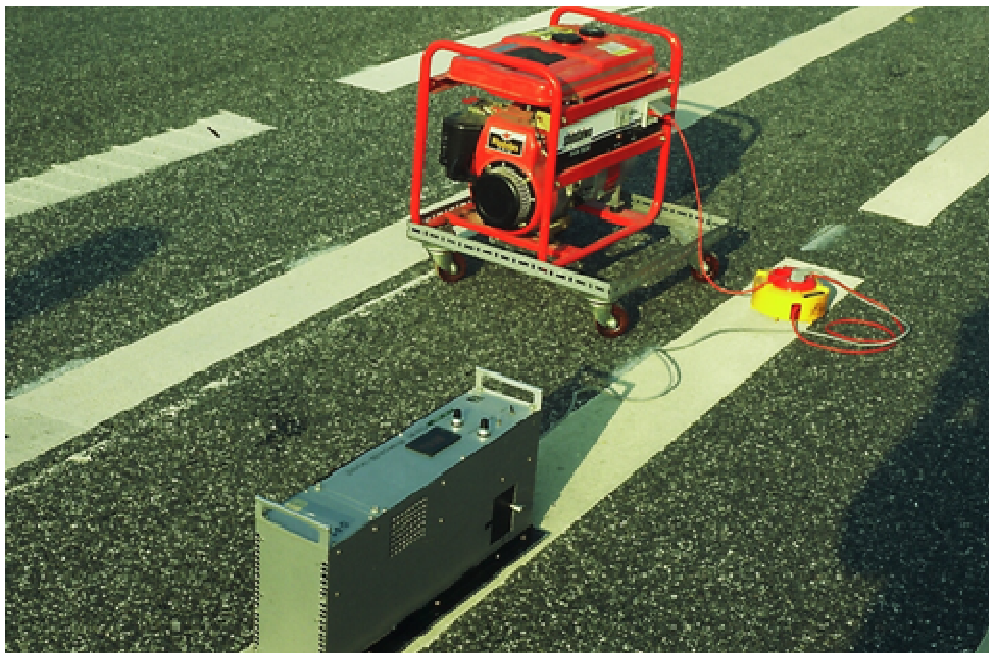
Figure D.6: An early type of retroreflectometer.
