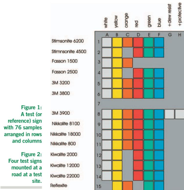
Figure 1: A test (or reference) sign with 76 samples arranged in rows and columns
