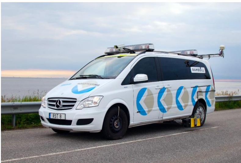
Figure 1. Mobile measurement system registering the retroreflectivity and profile of road markings.
